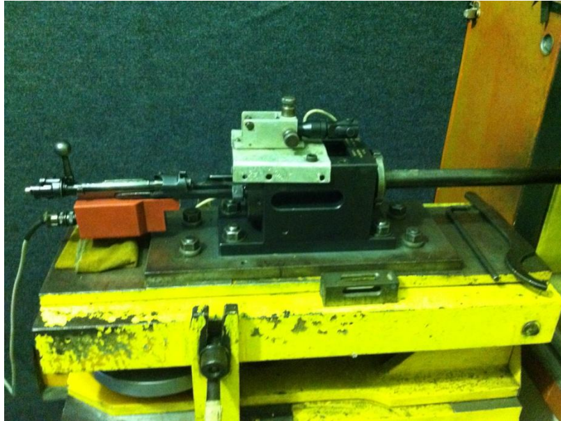
FIG. 3.4 Dispositivo de disparo B290 Ammunition Test Gun (HPI – High Pressure Instrumentation).
